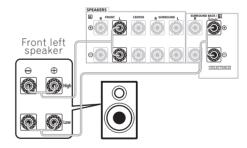
Since both front and surround back speaker terminals output the same audio, it doesn't matter which set (front or surround back) is powering which part (**High** or **Low**) of the speaker.
